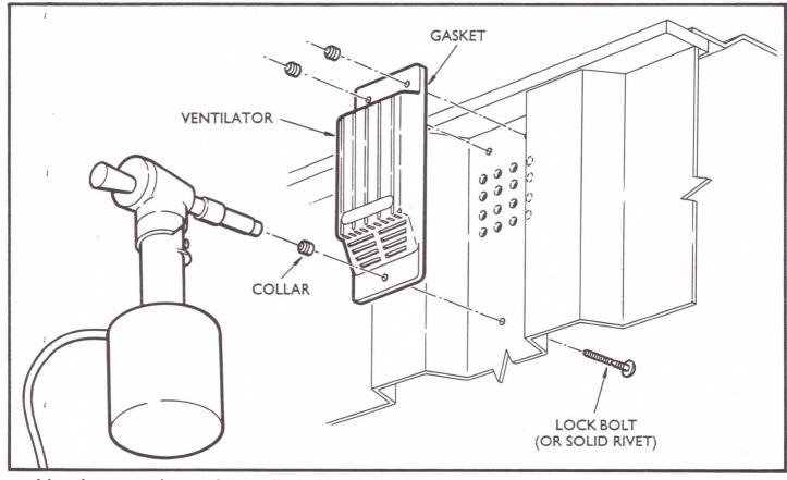
Ventilator can be easily installed. It can be dismantled for refurbishment and reinstalled.
