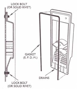
Triple internal baffle construction prevents rain or seawater from leaking into container.
